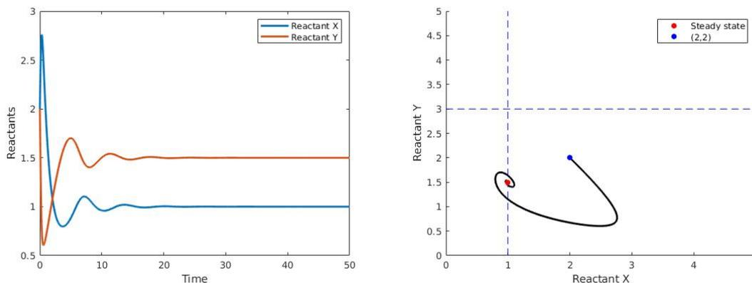
The trajectory of the variables  $x$  and  $y$  change in time so that they achieve the steady state values, 1 and 1.5, respectively, in an oscillatory way. The representation of phase space
