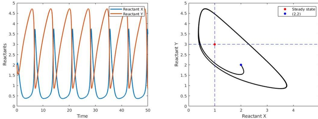
In this case, the trajectories are periodic both for  $x$  and  $y$ . As a consequence, the orbit in phase space is a closed orbit; therefore, it can be envisaged that its a limit cycle. This results are in agreement with the initial calculations of the steady states; in fact, the center of the limit cycle is  $(1,3)$
